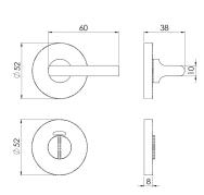
Thumbturn and Release on a concealed fix press on rose. The turn side has a long straight tubular bar, and the release side has a vacant/engaged indicator. Ideal for public/office toilet doors where a more ergonomic operation is a necessary requirement. Part of the Steelworx range in G201 Stainless Steel.
