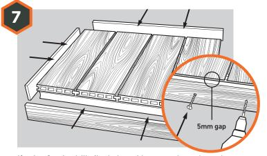
If using fascia, drill pilot holes with counterbore through the fascia at 200-300mm intervals. According to ambient temperature allow a **5-7mm gap** between end of deck board and the fascia. Screw fascia to the joist. Always screw fascia to the joist at a 90° degree angle.
