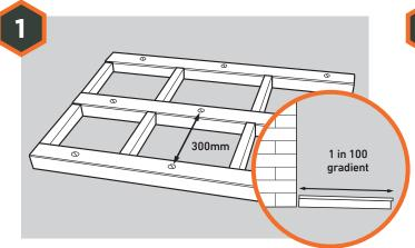
We recommend using treated 47x100mm timber joists and building in a gradual gradient of at least 1 in 100 (1%) that runs away from any adjoining buildings. Boards should run lengthways down this gradient to help water naturally disperse.
