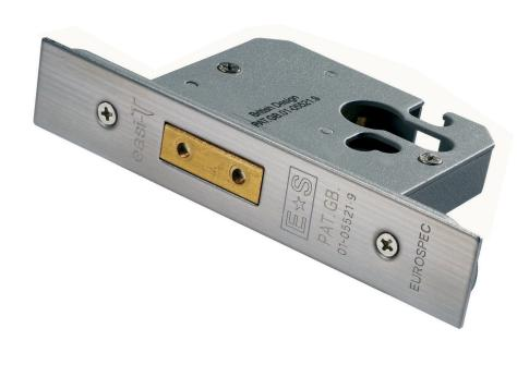
Euro Profile Deadlock in 64mm or 76mm option. Radius version also available. Certified to BS EN 12209 Lock used as a matter of course by the national house builders. This lock provides a good degree of security and carries a 10 year mechanical guarantee.
