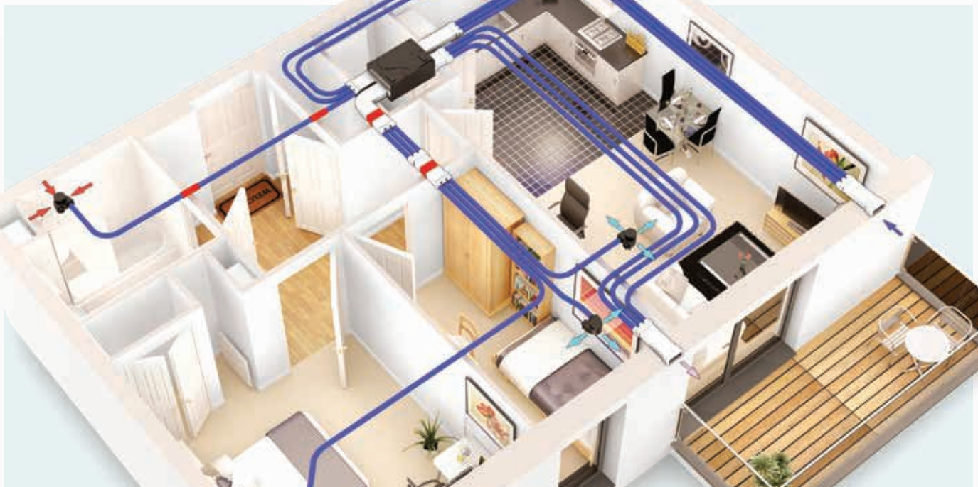
The property image illustrates how a typical Domus Radial system can be configured.
