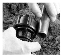
3. Witness Mark the Pipe To ensure the correct insertion depth witness the mark by lining up the pipe against the fitting and using the flange of the body as an indicator.
