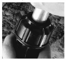
Fully Installed The fitting is fully installed when the nut butts against the flange of the body.
