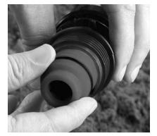
2. Position the Connection Kit Take the appropriate connection kit and place it in the body of the fitting with the tapered end pointing outwards.
