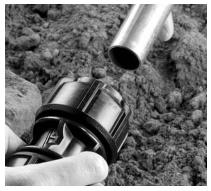
**2. Ready to Use Position** Prior to pipe insertion ensure the nut is fully relaxed and 2 threads are showing.
