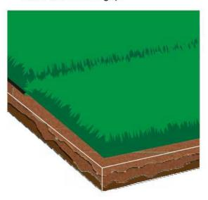
Peel the grass back and lay the joining tape under the join.
