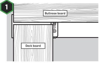
Insert the Universal Clip as shown in the diagram with the front of the clip positioned in the groove of the secured bullnose deck board.
