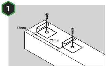
Place two starter clips as shown in the above diagram and secure in place with the respective screws. Ensure that the spacing measurements are correct.
