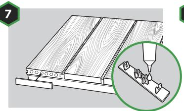
If using end caps, apply a high quality grab adhesive to the end caps to secure for extra adhesion. Wipe away any excess from the edge of the cap.
