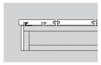
After installing the *HD Deck® Dual* bullnose deck board, as per the above instructions, use the Universal Clip to secure to the rest of the deck. See *Using the New Universal Clip* overleaf.
